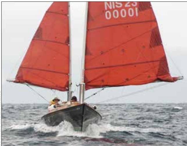
An interest in shoal draft and freestanding rigs led Kirby to design a line of sharpie-type small cruising boats to be built in plywood. He sold hundreds of plans for the home builder or professional, and in all produced five Norwalk Island Sharpie models ranging from 18' to 31' (5.5m to 9.5m).
